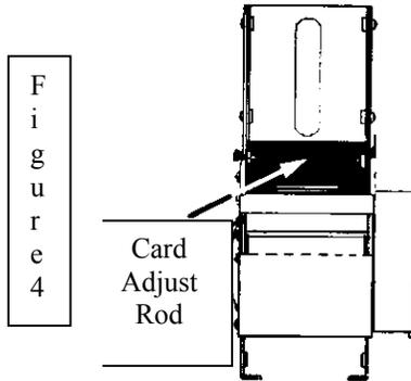
4. Using a #1 Phillips screwdriver, Turn the card adjustment rod located between the dispenser and the door. Clockwise to make the card size smaller, Counter-clockwise to make the card size thicker.
