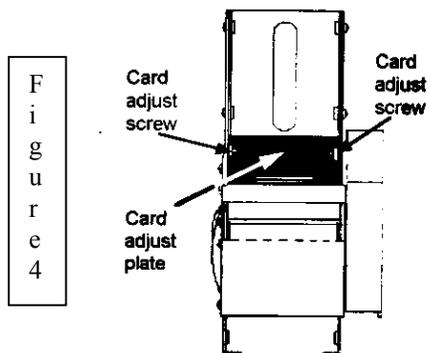
4. Using a #1 Phillips screwdriver, turn the set screw above the card adjustment arrow counter-clockwise.
